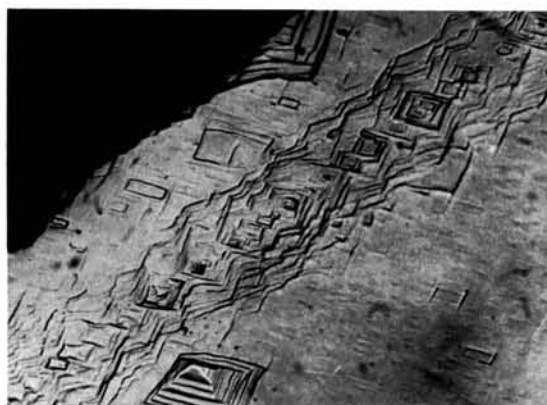
Fig. 10. An etch pattern showing a row of pits ( \times 130 ).
