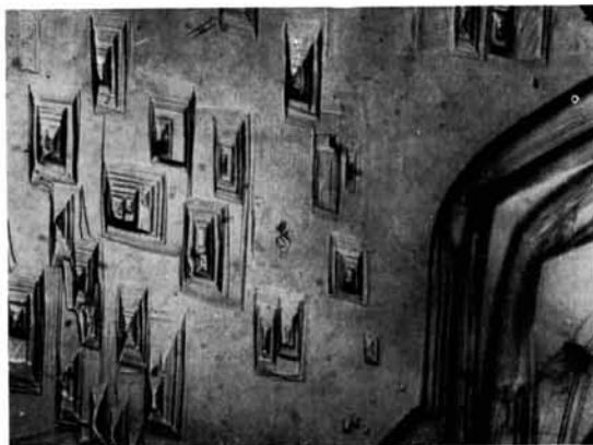
Fig. 3. Detail of part of a surface etched as in Fig. 2(a) ( \times 130 ).
